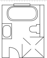
Removing an existing stud wall created more space for a new bath and a larger shower area. A smaller stud wall has been built to conceal pipework and provide storage
